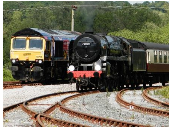
Britannia and 66718 together. The sun came out for days two and three of the event! This photo hints at the steep gradient down to Northbridge Street, as the 66 is on level track which is a couple of feet higher than the camera position. Each train was topped and tailed, in line with modern practice.
